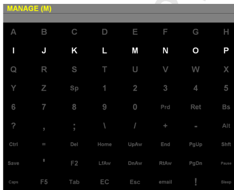
Fig. 2. P300 Speller matrix with example word to be spelled (“MANAGE”). At this moment, the subject is attending to flashes of the letter “M”; the row containing this character is currently illuminated. In “test” mode, after each row and column has flashed five times, the P300 Speller will select a character and display it in the row underneath the target word.
