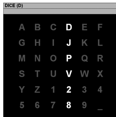
Fig. 1. The 6 × 6 matrix used in the current study. A row or column intensifies for 100 ms every 175 ms. The letter in parentheses at the top of the window is the current target letter “D.” A P300 should be elicited when the fourth column or first row is intensified. After the intensification sequence for a character epoch, the result is classified and online feedback is provided directly below the character to be copied.
