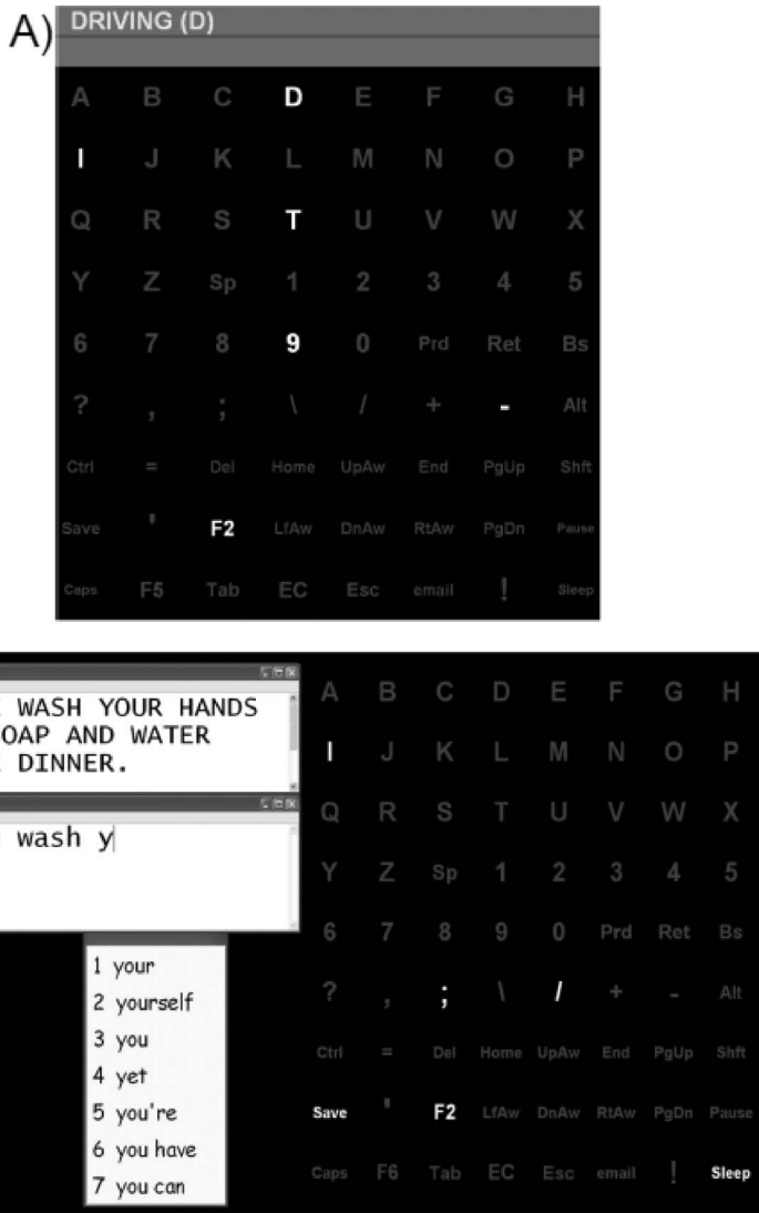
FIGURE 1 A) The 8 \times 9 matrix used during the calibration phase and online spelling phase of the experiment. In this example, the target item “D” is noted by the letter in parentheses at the end of the word. Participants are instructed to count the number of time the target item flashes. After all items have flashed a predetermined number of times, there is a 3.5-s pause in which the item in parentheses changes to the next letter of the word to indicate the next target item. B) The 8 \times 9 matrix and additional windows used during the online spelling phase of the experiment. Right: the flashing matrix used to make item selections. Left top: the sentence target window. Left middle: the sentence output window. Left bottom: the predictive spelling window used in the PS condition (see text for details).
